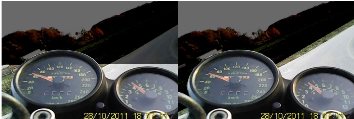
Picture 14: Illuminated part of a road with conventional (left) and adaptive (right) headlight
