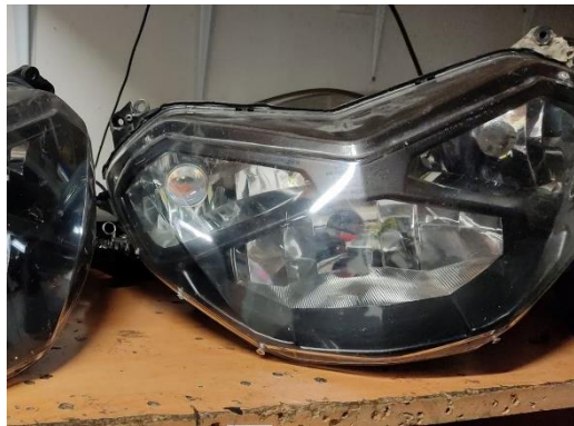
Picture 21: A modified headlight assembly of a motorcycle Aprilia RST 1000 Futura – there is a 1.8« LED projector that rotates and acts as an adaptive headlight seen in the left part of a picture
