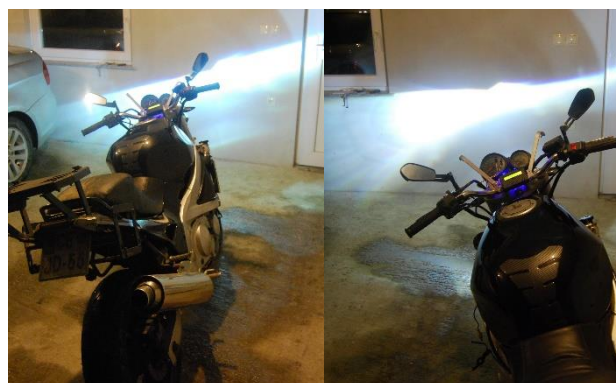
Picture 19: Version 1 with adaptive function off (left) and on (right)
